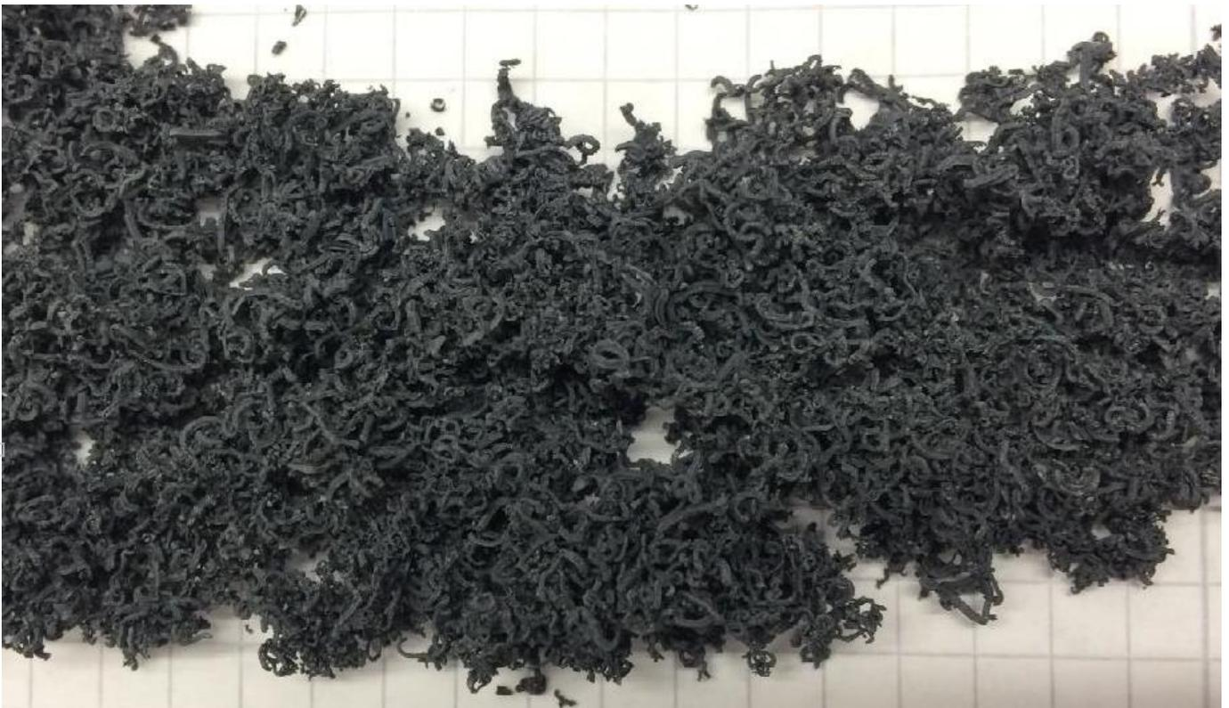
**Figure 1: Ancuabe T12 BF-3, 50 mesh graphite concentrate, converted to expanded graphite**
